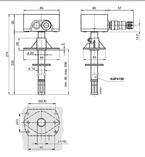
Drilling template with (without) mounting flange
