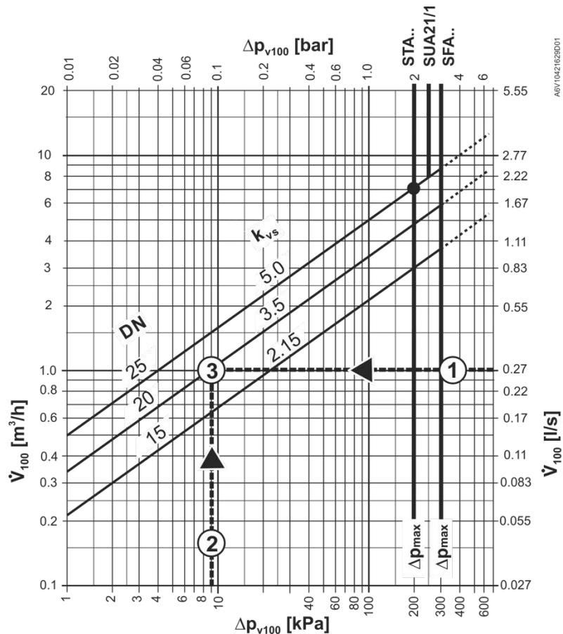
$\Delta p_{v100}$  = Differential pressure across the fully open valve and the valve's control path A → AB (2-port valves), AB → A (3-port diverting valves) by a volume flow  $\dot{V}_{100}$
